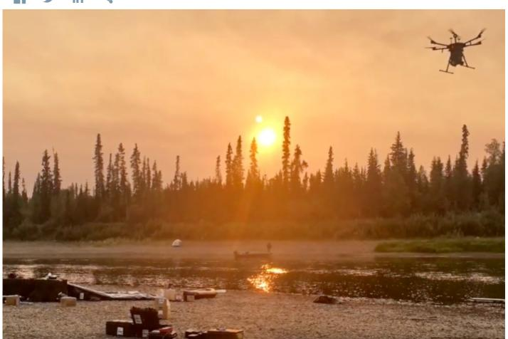
Drone Amplified is headed by Carrick Detweiler, University of Nebraska-Lincoln associate professor of computer science and engineering. The company's drone-mounted technology carries chemical spheres the size of ping pong balls. At the press of a button, the spheres drop and ignite — intentionally sparking small fires that burn vegetation and starve incoming wildfires of potential fuel.
